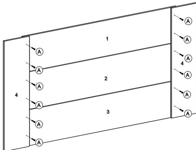
PARAFUSE O PAINEL E O SARRAFO TRASEIRO NOS PAINÉIS FRONTAIS
